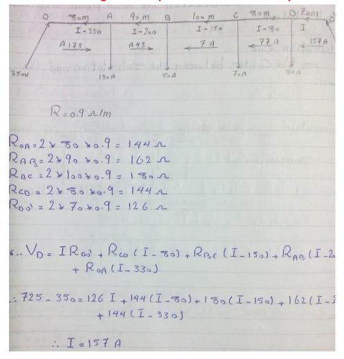
Vo = Ros \* Ios = 126 x 157 = 19782 V VDC = Rco x Ico = 144 x 77 = 110 50 V Vosc = RBC \* IBC = 180 \* 7 = 1260 v VOR = RAB \* IAB = 162 \* -43 = - 6966 V VDa = R.A + IOA = 144 + -173 = -24912 V · VD= Vo - VD0 = 725 - 19782 = - 19057 V Vc = VD - VD = - 19057 - 11088 = - 301451 VB = VC - VDBC = -30145 - 1260 = -31405 V VA = VB - VDAB = - 31405 - (-6966) = -24439 Pip Pip=(725\*157)+(350 x-173) = 53275 W
