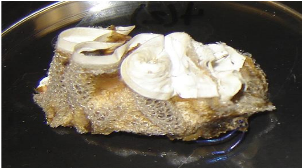
Fig.13: An explanted mesh consisting of a heavyweight polypropylene–ePTFE composite, after cleaning. This specimen is notable for the contraction of the mesh, which led to exposure of the polypropylene to the viscera (Bachman and Ramshaw, 2008).
