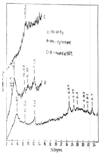
Fig@gy-ray diffraction pattern of clay fraction profile No7 - depth 50-80 cm
