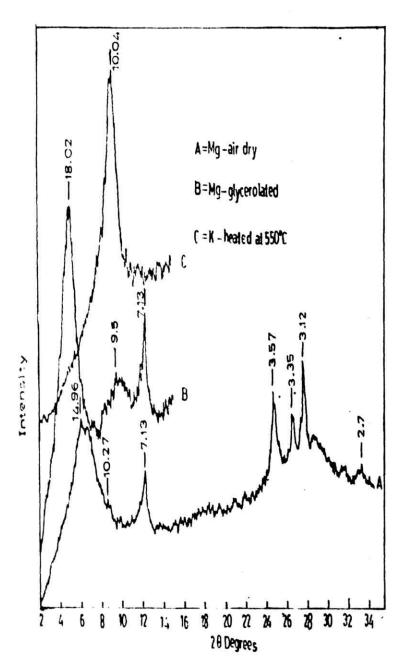
Fig(a) x-ray diffraction pattern of day fraction profile No.8 - depth 20-40 cm
