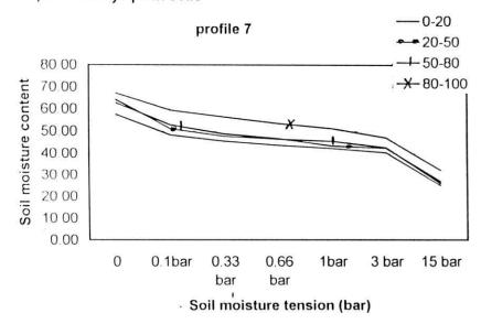
Fig ( 13 ) Moisture characteristic curvesof profile (7) at VA1 soil mapping unit, El-Hasainiya plain soils
