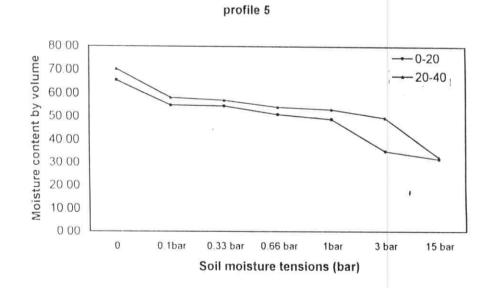
Fig ( 11 ) Moisture characteristic curves profile (5) at VA1 soil mapping unit El-Hasainiya plain soils
