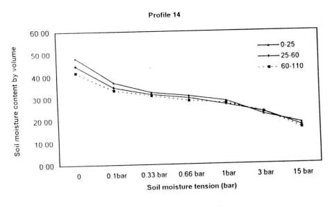
Fig (21) Moisture characteristic curvesof profile (14) at AV soil mapping unit ,EI-Hasainiya plain soils
