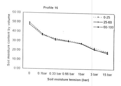
Fig (23) Moisture characteristic curve of profile (16 at AV soil mapping) unit, El-Hasainiya plain soils
