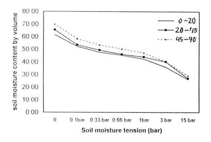
Fig ( 12 ) Moisture characteristic curvesof profile (6) at VA1 soil mapping unit, El-Hasainiya plain soils
