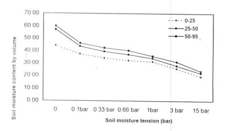
Fig ( 18 ) Moisture characteristic curvesof profile (11) at VT soil mapping unit, El-Hasainiya plain soils
