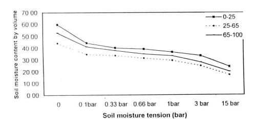
Fig ( 17 ) Moisture characteristic curves f profile (18) at VA2soil mapping unit, El-Hasainiya plain soils
