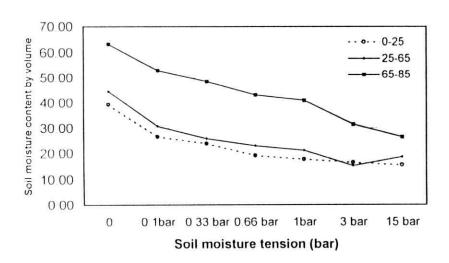
Fig ( 16 ) Moisture characteristic curvesof profile (4) at VA2 soil mapping unit ,EI-Hasainiya plain soils
