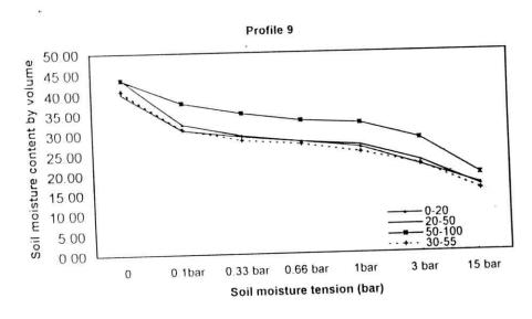
Fig ( 25 ) Moisture characteristic eurvesof profile (9 at AT soil mapping) unit , El-Hasainiya plain soils
