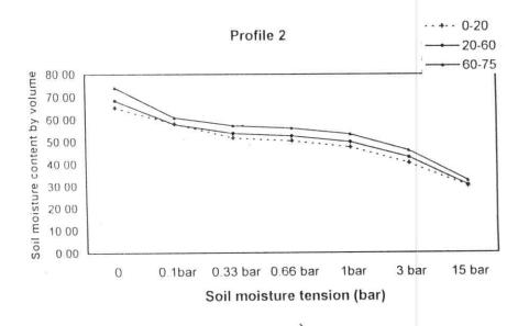
Fig ( 15 ) Moisture characteristic curvesof profile (2) at VA2soil mapping unit, El-Hasainiya plain soils
