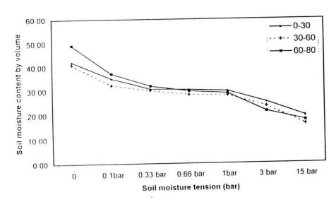
Fig (20) Moisture characteristic curvesof profile (13) at AV soil mapping unit ,EI-Hasainiya plain soils
