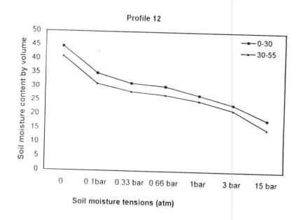
Fig ( 26 ) Moisture characteristic curves of the studied soils profile (12) at AT soil mapping unit
