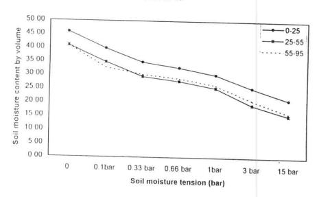
Fig ( 22 ) Moisture characteristic curves of profile (15) at AV soil mapping unit , El-Hasainiya plain soils
