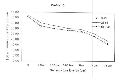
Fig ( 19 ) Moisture characteristic curves of profile (10) at AV soil mapping unit, El-Hasainiya plain soils
