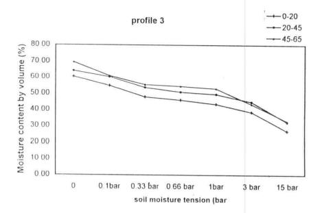
Fig ( 10 ) Moisture characteristic curvesof profile (3) at VA1 soil mapping unit ,EI-Hasainiya plain soils
