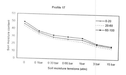
Fig ( 27 ) Moisture characteristic curvesof the studied soils profile (17) at AT soil mapping unit
