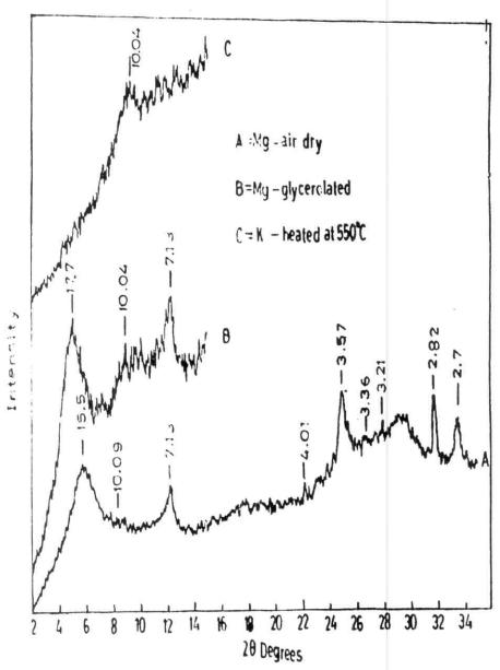
Fig(s2) x-ray diffraction pattern of clay fraction profile No.8 - depth 40-90 cm
