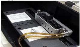
Temperature-controlled <u>cuvette</u> holder in a spectrophotometer.
