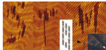
Letters "STM" written on the assembly of molecules bound by hydrogen bonding
