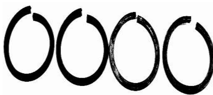
Unirradiated NBR o-ring seals after the tensile test (From the left to right: NO, NA, NB, and NC).
