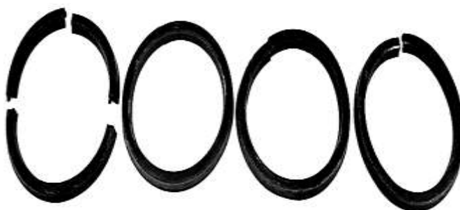
Irradiated NBR o-ring seals at 5 MGy after the tensile test (From the left to right: NO, NA, NB, and NC).
