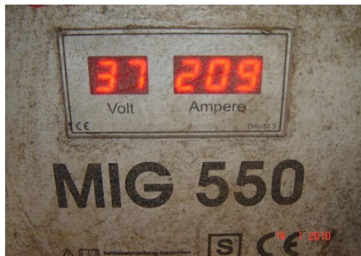
Fig (1-1): Measured volt and ampere during the welding process in the gas metal arc welding (GMAW) machine
