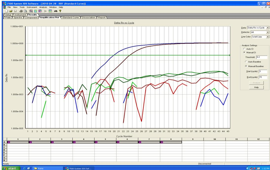
**Figure (1):** The real-time detection of the specific PCR products by fluorescence (y axis) (F1 detection wavelength or F1/F2 ratio) dependent on the PCR cycle number (x axis).
