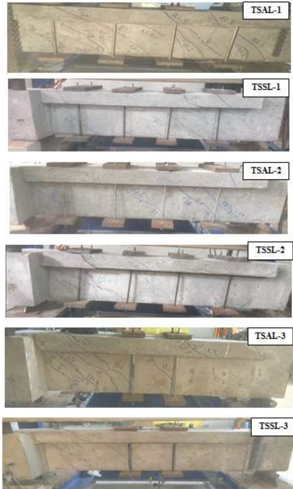
Fig. 6: (a) the crack pattern and failure modes for tested beams
