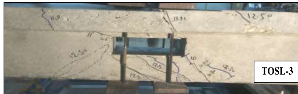
Fig. 6: (d) the crack pattern and failure modes for tested beams
