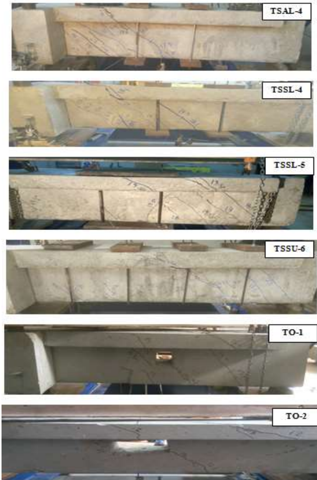
Fig. 6: (b) the crack pattern and failure modes for tested beams
