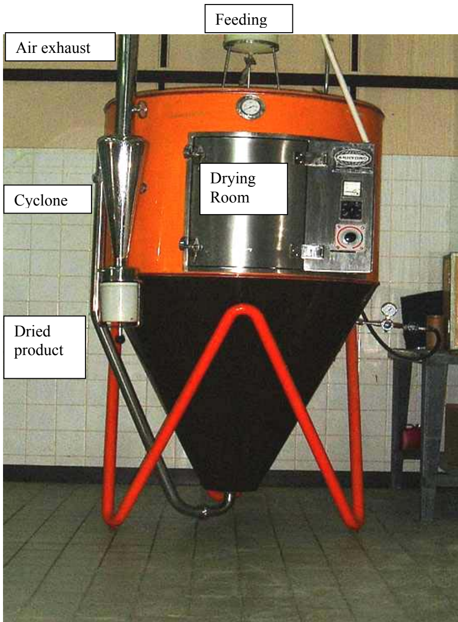
Figure 1a: Photograph of the lab-scale spray dryer.
