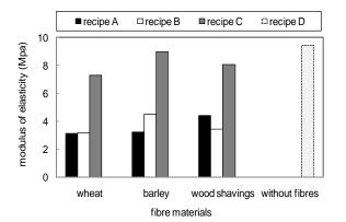
Fig14. Modulus of elasticity for the different treatments at failure condition
