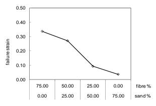
Fig 6. Failure strain for plaster reinforced with wood shavings fibers
