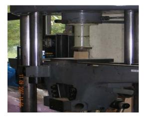
Fig 2. Compression test instrument
